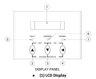
This Indicates the UPS operation information, including UPS status, input/output voltage, input/output frequency, battery voltage, battery capacity left, output load, inside temperature, and the times of history events. Besides, UPS output voltage and output frequency can be set from the LCD panel.
