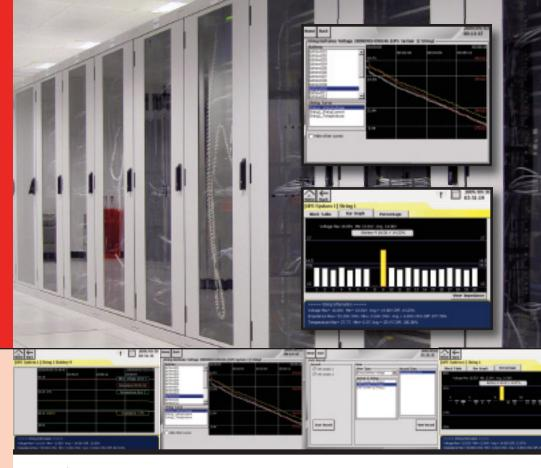
Perfect Power Systems Battery Tracker is designed to protect and enhance your investment in backup emergency power systems. Utilizing state of the art electronic "ohmic value" testing and monitoring, the Battery Tracker provides the added assurance that when emergencies happen, the power will be available when it's needed.
